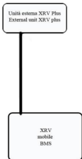
Systems with all indoor units series 4 and outdoor units series XRV Plus : connect the bus X-Y-E as shown in Fig 2/1
