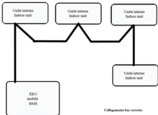
Systems with indoor units series 1 or 2 : connect the bus to the indoor units as shown in Fig. 2
